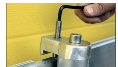
4 On top of the compression post retainer, turn the 12mm cap screw, clockwise, by hand, until finger tight.
