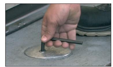
4 Using the 10mm Allen Key, turn the 12mm cap screw anti-clockwise until the top compression block can be removed.
