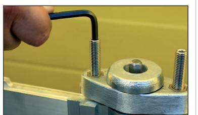
7 Using the 5mm Allen Key, turn each grub screw, clockwise, one full turn (360 degrees).
