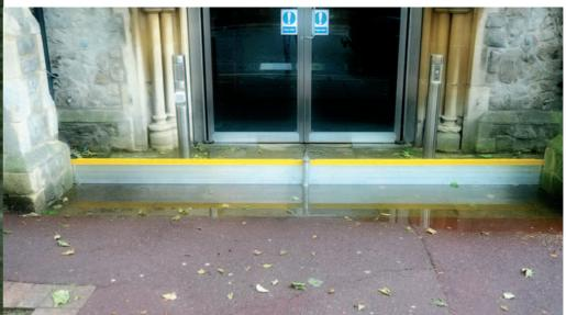
Suitable for installation on both residential and commercial property, Nautilus® 200 makes use of two permanently-fixed vertical side channels fitted either side of the opening to be protected, along with pre-installed unobtrusive ground fixtures to allow the Patented Twist and Lock post system (Patent No. 2371068) to be put in place.
